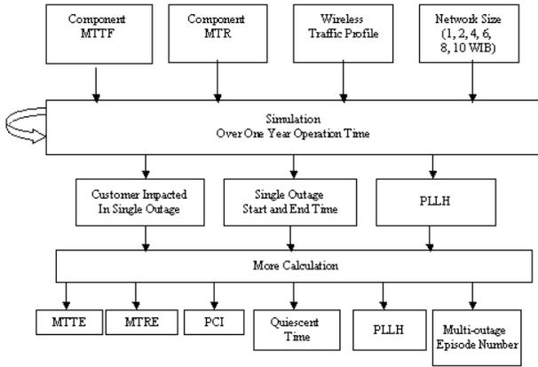
Figure 9. Process of Simulation and Results
