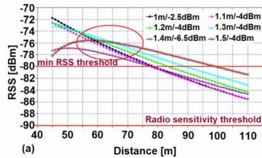
Figure 16. Non-neighbor interference simulations for square grid scheme
