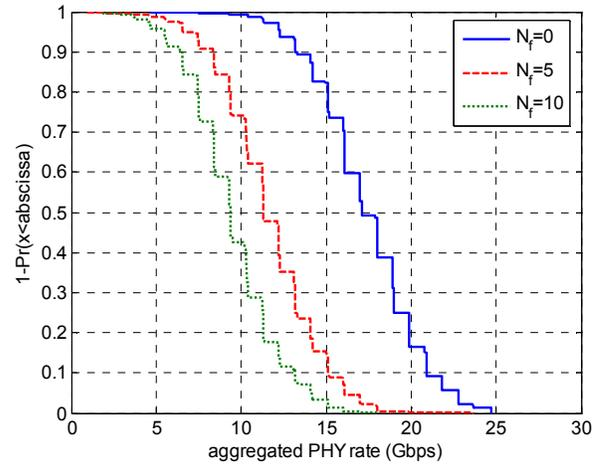
Fig. 16. Distribution of the aggregated PHY rate of the 1<sup>st</sup> hop links between the stations and the 60 GHz APs for the two-hop mesh (the stations with 4x4 square array antenna and the APs with 6x6 square array antenna)
