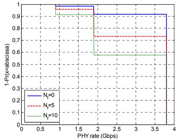
Fig. 15. Distribution of the PHY rate of the 2<sup>nd</sup> hop link between one of the 60 GHz AP and the combo-AP for the two-hop mesh (all the APs using the 6x6 square array antenna)
