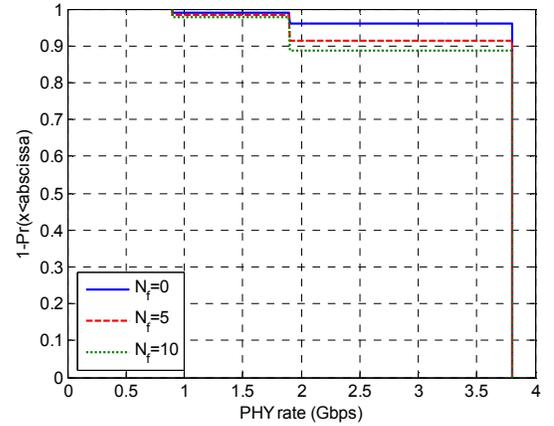
Fig. 9. Distribution of the PHY rate of the 2<sup>nd</sup> hop link between one of the 60 GHz AP and the combo-AP for the two-hop mesh (all the APs using the 6x6 square array antenna)
