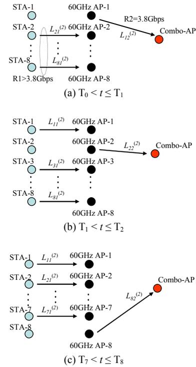
Fig. 11. Illustration of the two-hop mesh operation over the time  $T_0 < t \leq T_8$  achieving the end-to-end throughput close to the maximum PHY rate of the 2<sup>nd</sup>-hop link
