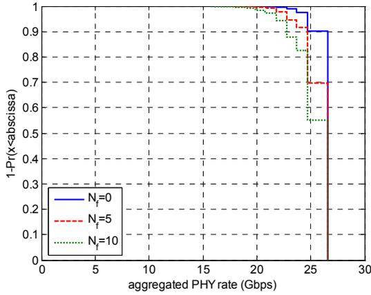
Fig. 10. Distribution of the aggregated PHY rate of the 1<sup>st</sup> hop links between the stations and the 60 GHz APs for the two-hop mesh (all the stations and the APs using the 6x6 square array antenna)
