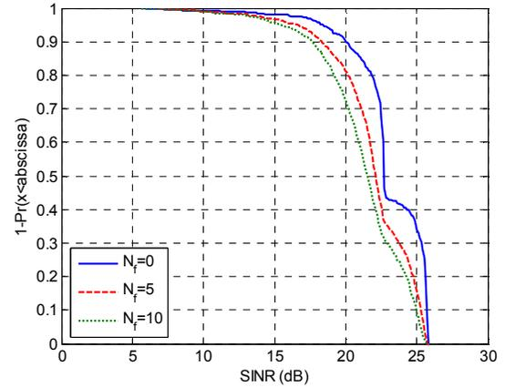
Fig. 8. Distribution of the SINR of the 2<sup>nd</sup> hop links between one of the 60 GHz AP and the combo-AP for the two-hop mesh (all the APs using the 6x6 square array antenna)
