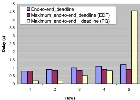
Figure 19. Measured maximum end-to-end deadline with EDF and PQ
