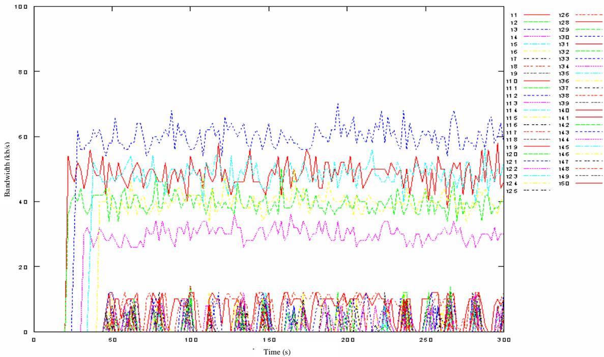
Figure 10. Measured instantaneous bandwidth for 6 QoS and 44 BE flows
