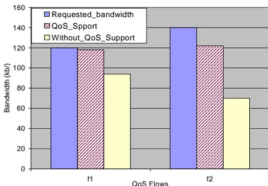
**Figure 23.** Measured average bandwidth for QoS flows in the two cases: in presence and in absence of QoS support
