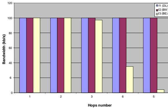
Figure 16. Measured average bandwidth according to hops number
