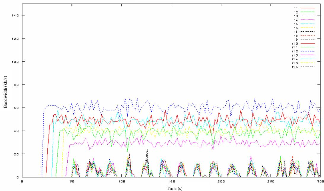
**Figure 8.** Measured instantaneous bandwidth for 6 QoS flows and 10 BE flows
