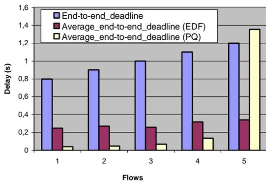
Figure 18. Measured average end-to-end deadline with EDF and PQ
