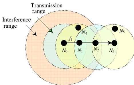
Figure 1. Interference phenomenon
