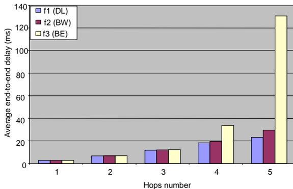
Figure 17. Measured average end-to-end delay according to hops number
