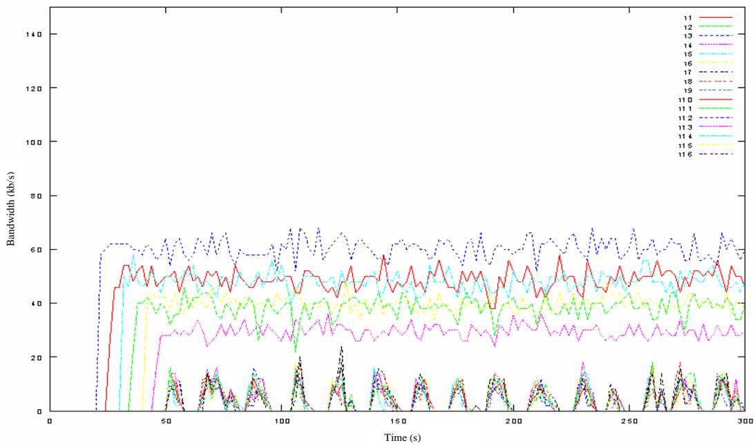
**Figure 15.** Measured instantaneous bandwidth with QoS support
