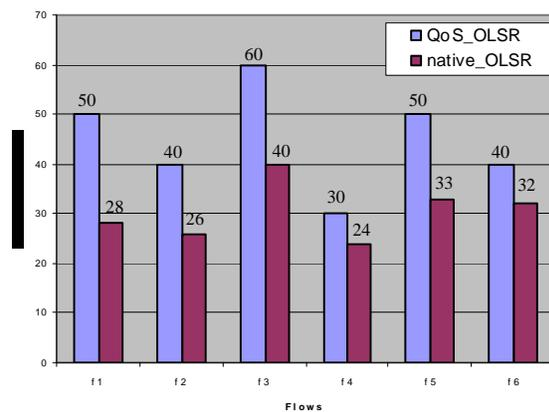
Figure 13. Average measured bandwidth of QoS flows with QoS OLSR and native OLSR
