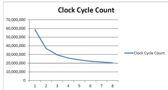
Figure 7. Performance Test (clock cycles / no of cores).
