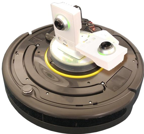
Fig. 10. Prototype configuration based on a vacuum cleaning robot.
