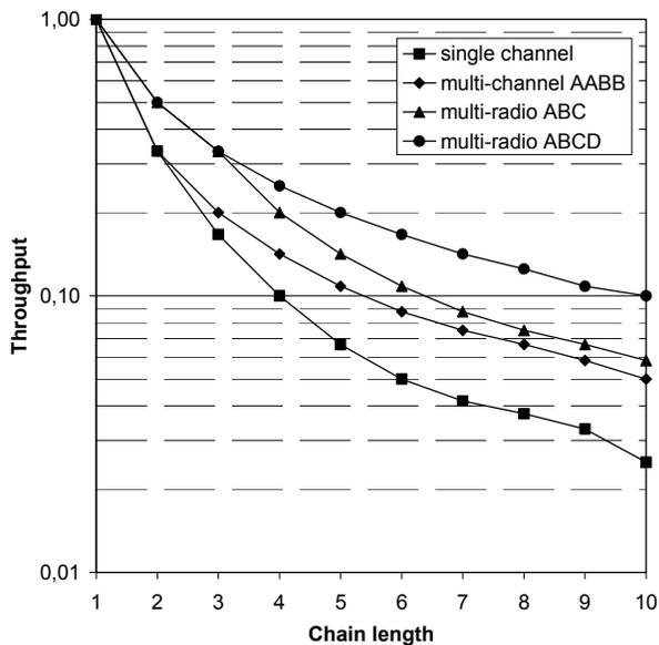
Fig. 21 Comparison of selected multi-channel and multi-radio configurations of the 802.16 WMN.
