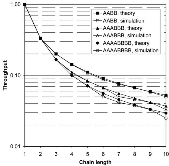
Fig. 9 2-channel configuration – comparison of 3 possible channel assignment schemes.
