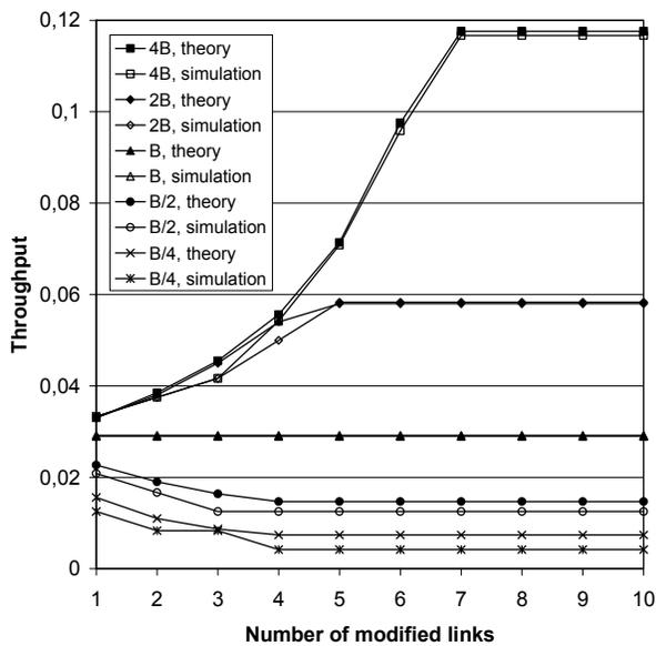
Fig. 7 Effect of adaptive coding and modulation – throughput vs. number of affected links in the chain.
