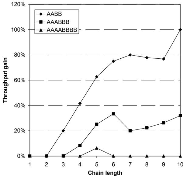
Fig. 10 Throughput increase (relative to the single channel) for the channel assignments shown in Fig. 9.
