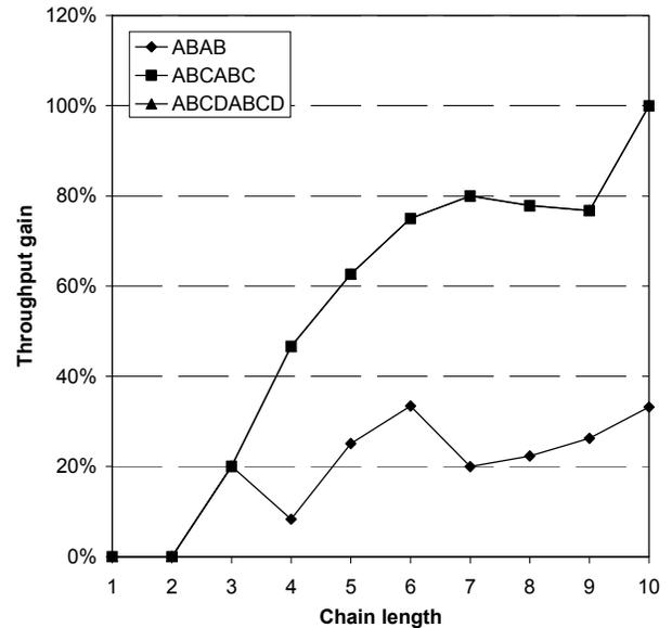
Fig. 12 Throughput increase (relative to the single channel) for the channel assignments shown in Fig. 11
