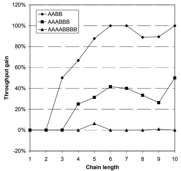
Fig. 16 Throughput increase (relative to the single channel) for the channel assignments shown in Fig. 15.
