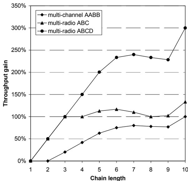
Fig. 22 Throughput increase (relative to the single channel) for the channel assignments shown in Fig. 21
