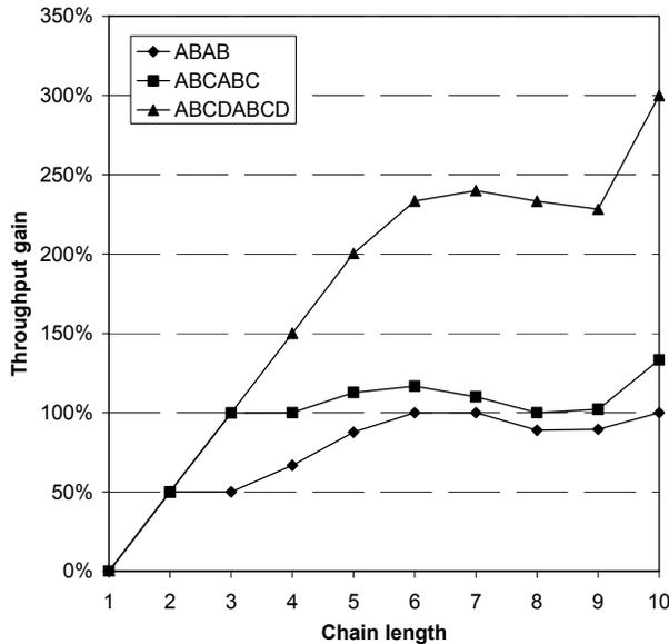
Fig. 18 Throughput increase (relative to the single channel) for the channel assignments shown in Fig. 17.
