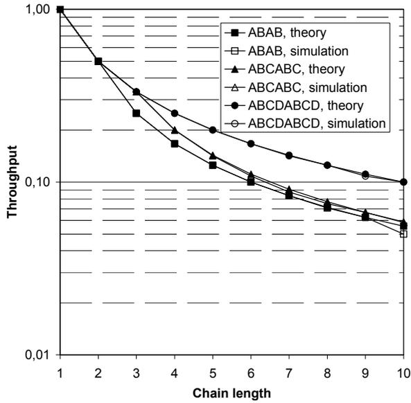
Fig. 17 Comparison of 2, 3 and 4 channel configurations with multi-radio nodes.
