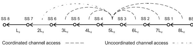
Fig. 2 Simple chain topology of WMN with 8 nodes.
