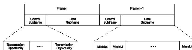
Fig. 1 IEEE 802.16 mesh mode frame structure.
