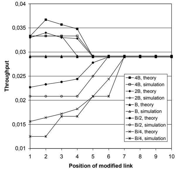
Fig. 8 Effect of adaptive coding and modulation – throughput vs. position of affected link in the chain.
