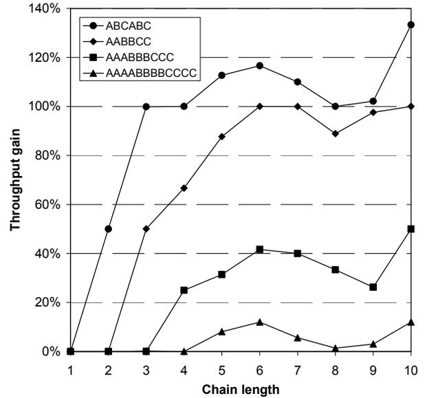
Fig. 20 Throughput increase (relative to the single channel) for the channel assignments shown in Fig. 19.
