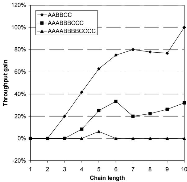
Fig. 14 Throughput increase (relative to the single channel) for the channel assignments shown in Fig. 13
