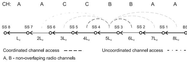
Fig. 4 Simple chain topology of WMN with 8 multi-radio nodes.
