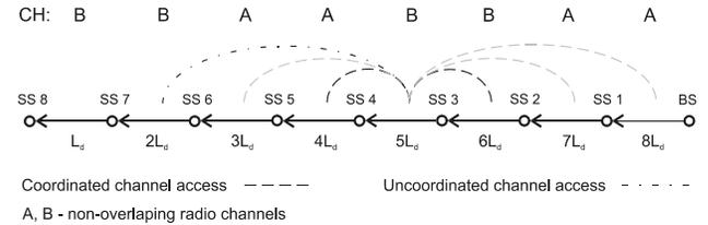
Fig. 3 Simple chain topology of WMN with 8 nodes configured in multi-channel mode.
