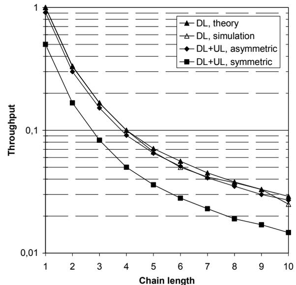
Fig. 6 Throughput vs. number of downloading nodes, unidirectional and bidirectional traffic.
