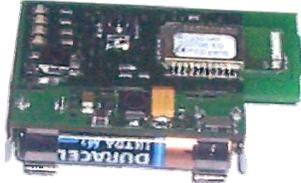
**Fig. 16. ZigBee-ready Temperature Sensor Node**
