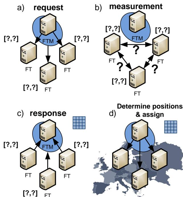
Fig. 2. Hierarchical aggregation scheme with many feedback targets.
