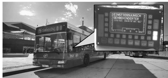
Figure 7. Bus driver display shows requested assistance
