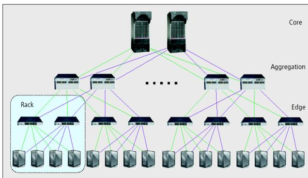
Figure 3. Typical network topology of a data center [9].
