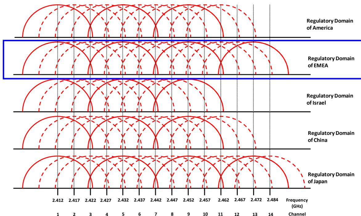
Figure 25. Channels in the frequency band of 2.4 GHz
