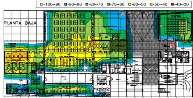
Figure 6. Radio coverage map of the ground floor for UPVNET2G
