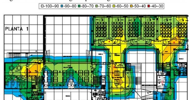
Figure 8. Radio coverage map of the first floor for UPVNET.
