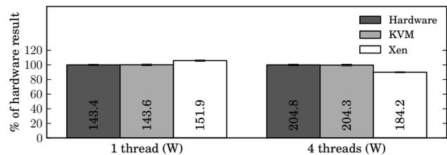
Figure 6. Power consumption under high CPU load with BurnInSSE
