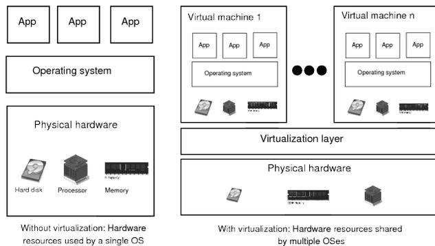
Figure 1. A non-virtualized and a virtualized system
