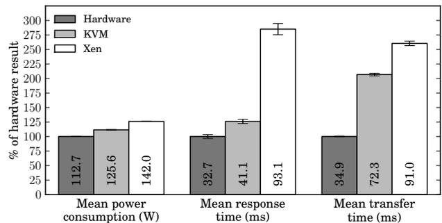
Figure 10. Power consumption and Httpperf results of different virtualization solutions
