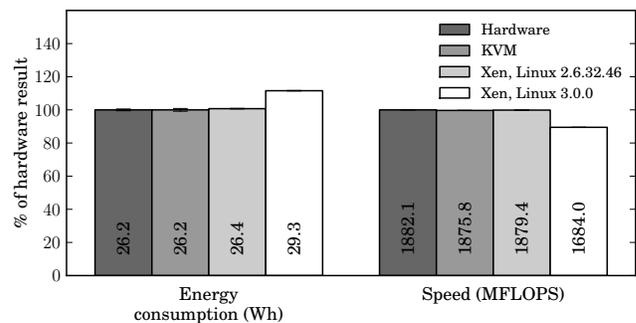
Figure 7. Energy consumption under high CPU load with Linpack
