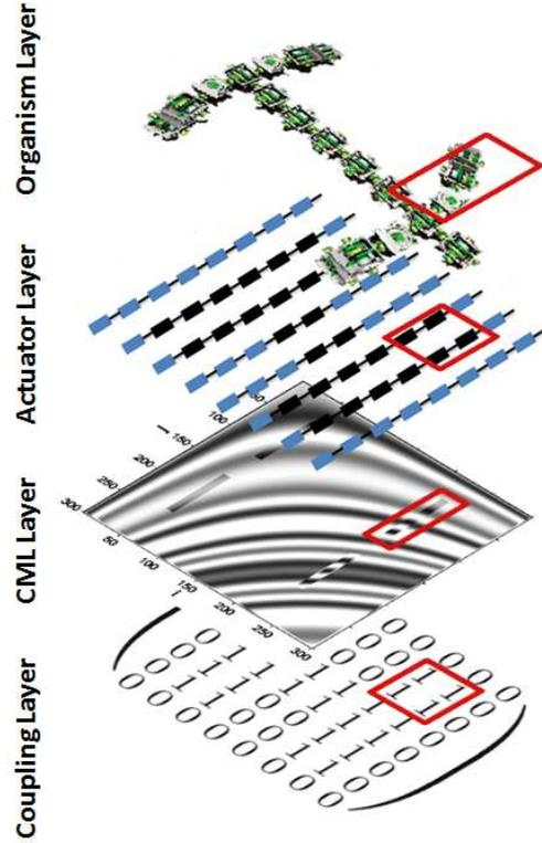
Figure 17. Architecture of Active Phase Perturbation Approach for Locomotion. This figure demonstrates how the CML based approach can directly refer to real robotic applications.
