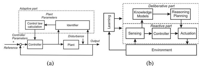
Figure 3. A high-level architecture for (a) adaptive control (b) adaptive behavioral systems (images from [14]).
