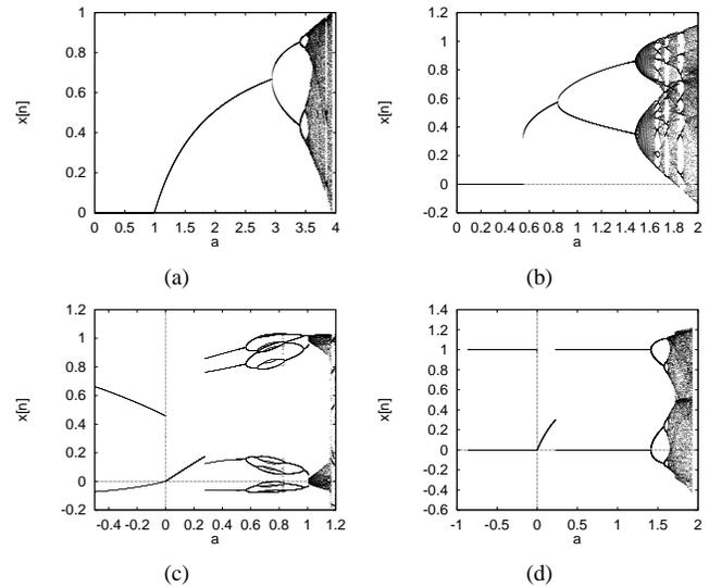
Figure 11. Several examples of qualitatively different types of behavior of the system (1). Bifurcation diagrams of the OLL map (1) at parameters: (a)  $b = 1, c = 0.1, x_0 = 0.1$ ; (b)  $b = 2, c = 0.6, x_0 = 0.4$ ; (c)  $b = -1.5, c = -1, x_0 = 0.1$ ; (d)  $b = -0.5, c = -1, x_0 = 0.1$ .
