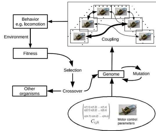
Figure 19. Evolutionary Concept: The genome contains the coupling matrix and parameter of the robot organism. This genome can be evolved over time and thus affects the behavior, respectively adapts the behavior. Through environmental and local feedback, the current fitness can be measured and optional crossover operators with other organisms can be applied.
