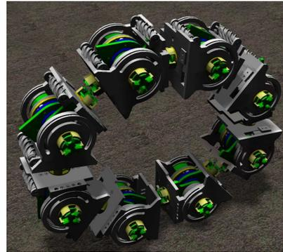
Figure 12. Multi-robot organism connected to a ring.
