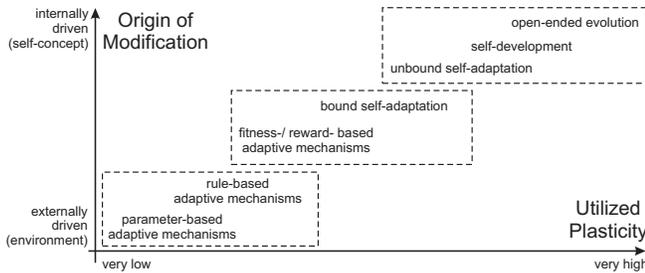
Figure 7. Three groups of adaptive and self-adaptive mechanisms placed along the used degrees of plasticity and origin of modification.
