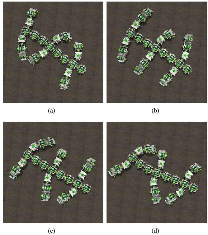
Figure 8. Top-down view on a hexapod multi-robot organism from Figure 9(a). Shown are four different positions of legs to illustrate a complexity of collective locomotion.
