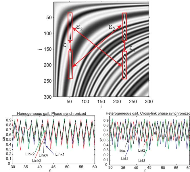
Figure 18. Time evolution of non-coupled (left image) and coupled (right image) sites in the activated areas for the four main links of the robot organisms. Coupling parameter are:  $\epsilon_1 = -0.01$  and  $\epsilon_2 = -0.001$ . When system gets synchronized it can be observed that links one and four (blue and black lines) as well as the links two and three (red and green lines) get synchronized crosswise.
