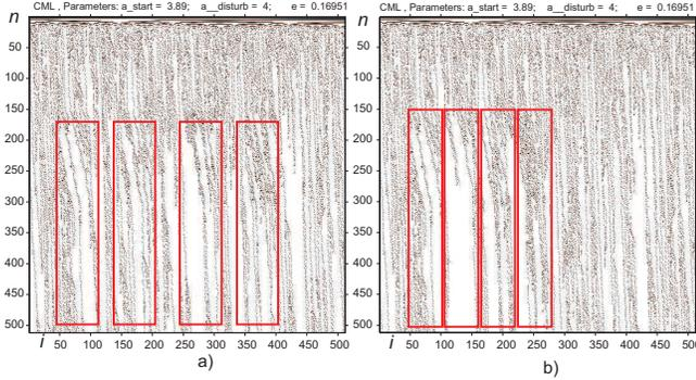
Figure 13. One-way coupled map lattice. Initial conditions:  $x_1^i = 0.1 + 0.0000049i$ . Boundary conditions:  $x_1^i = x_m^i$ ; (a) disturbances (i.e. motor voltage drops) are simulated in a large distance and do not significantly affect each other; (b) disturbed sites are in local range and affect more each other than in (a).
