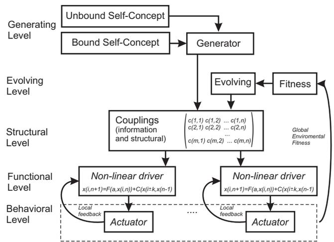
Figure 10. Different levels of adaptive collective locomotion.
