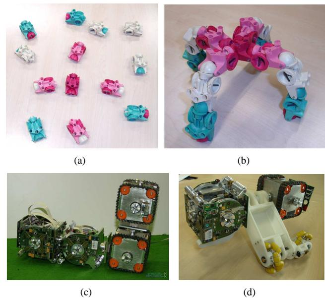
Figure 1. (a) Prove-of-concept: individual robots; (b) Prove-of-concept: aggregated robots into an artificial organism; (c), (d) Real prototypes: aggregated robots (images ©SYMBRION, REPLICATOR projects).
