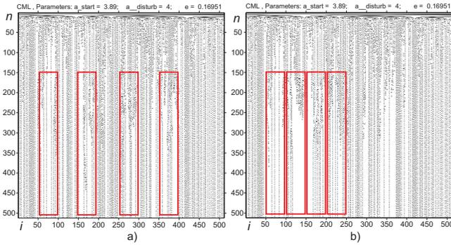
Figure 14. Two-way coupled map. Initial condition:  $x_1^i = 0.1 + 0.0000049i$ . Boundary condition:  $x_1^i = x_m^i$ ; (a) disturbances are simulated in a large distance and do not significantly affect each other; (b) disturbed sites are in local range and affect more each other than in (a).
