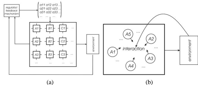
Figure 4. Simplified structure of (a) modularity-based adaptive mechanisms ; (b) self-organized adaptive mechanisms.
