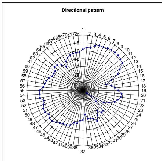
Figure 9. The directional pattern of the DA unit. The reference level 0 dB corresponds to an RSSI of -50 dBm.
