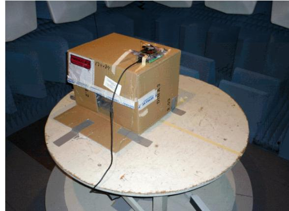
Figure 8. The ZigBee network device on the electrically rotatable measurement table.
