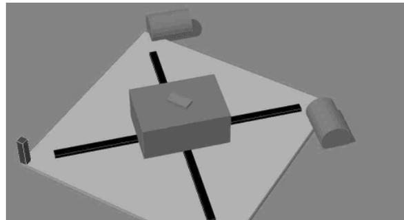
Figure 4. DA realised with two motors pulling a sledge against springs. The sledge has a servo for braking and an antenna element on it.
