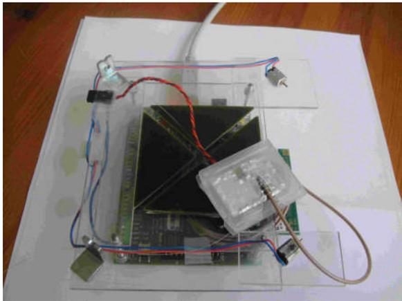
Figure 5. The DA antenna construction on Dresden RCB. The two motors are visible. The servo for the braking function is underneath the board which has the X-shaped hole.
