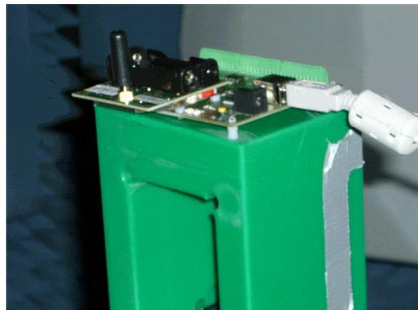
Figure 7. The ZigBee coordinator radio in the anechoic chamber.
