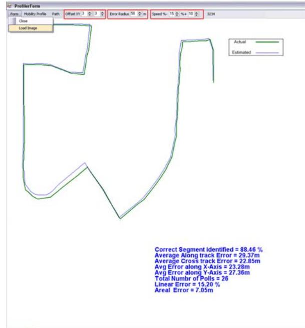
Figure 26. Mobility profiling simulator's GUI, the trajectory estimation window.
