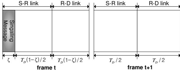
Figure 3. The frame structure of the proposed scheduling
