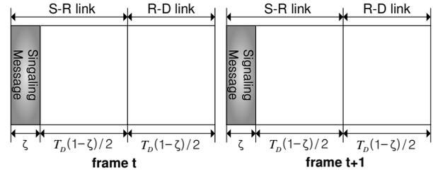
Figure 2. The frame structure of the conventional scheduling
