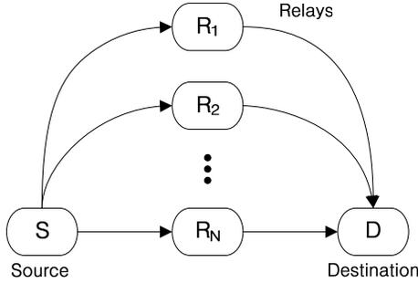
Figure 1. The multi-relay network
