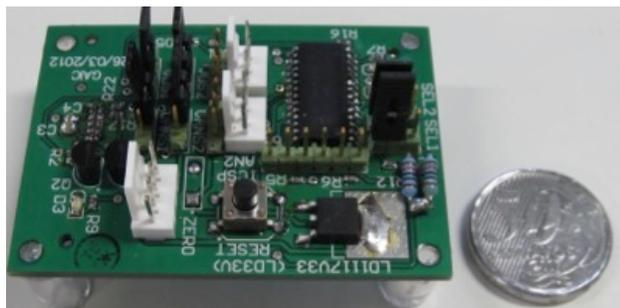
Figure 4. Intelligent Sensor Module (ISM).
