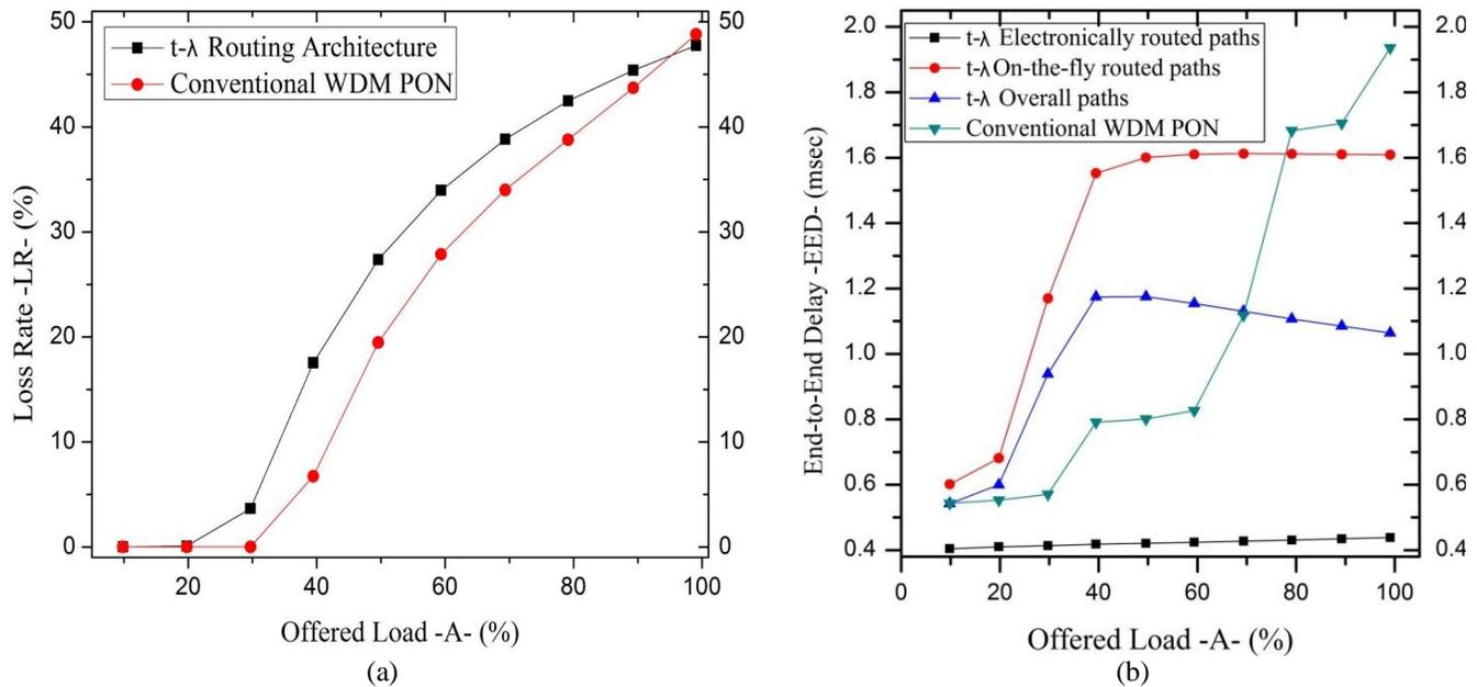
Figure 3. Simulations Results for 70% of A (Offered Load) destined to Metro Node (MN).
