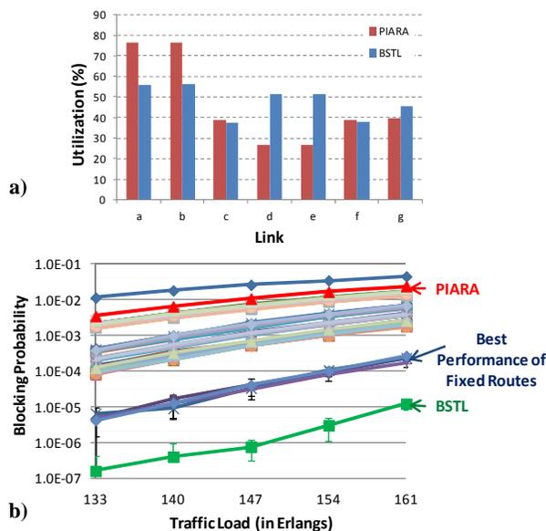
Figure 5. Link Utilizations (a) and Blocking Probabilities (b) for BSTL and PIARA algorithms in the scenario R6NNTL/IT=2.
