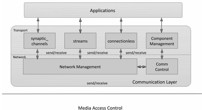
Figure 4. The architecture of the Communication Layer
