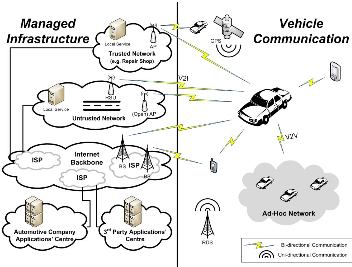
Fig. 1. Model of the connected car infrastructure
