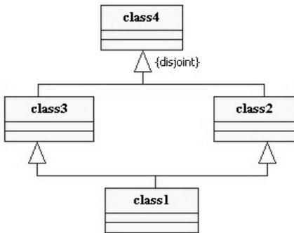
Figure 3. Inconsistent Class Diagram
