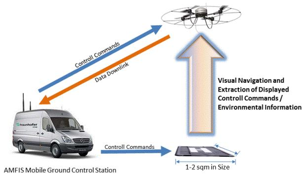
Figure 1. Sktech of the final target system.
