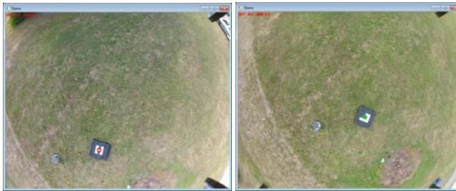
Figure 4. In-flight detection of shape "H" and "L" marked by colored circles at the center of the pattern ("H" is marked red; "L" is marked green)
