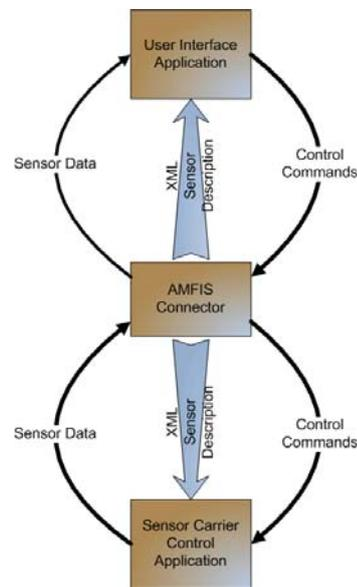
Fig. 3 Architecture of the AMFIS Framework.
