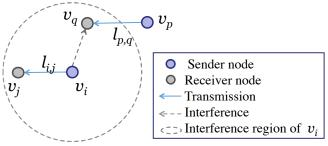
Figure 3. Radio wave interference model
