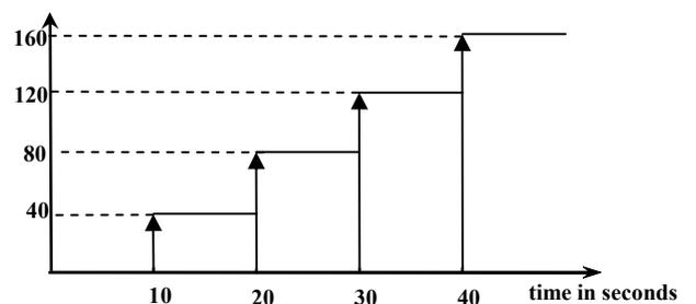
Figure 8. Total Bandwidth Allocation for Current Method
