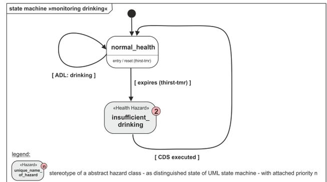
Figure 4: Simple state machine for concluding about the health hazard resulting from insufficient liquid ingestion
