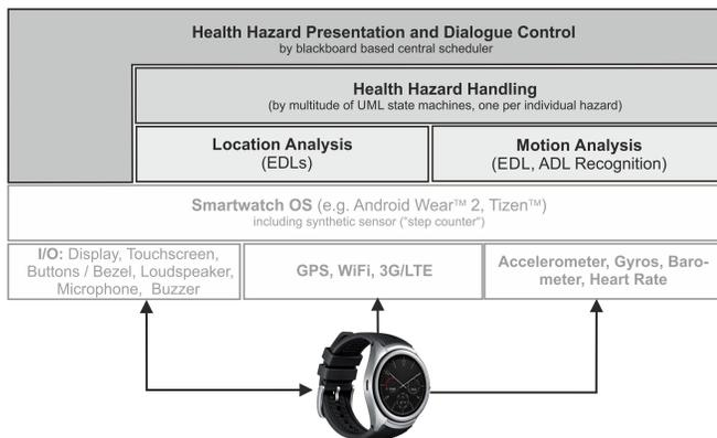
Figure 3: Block diagram of the smartwatch app
