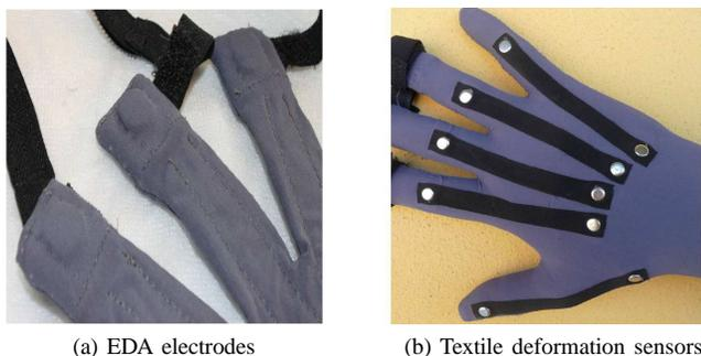
Fig. 1: Multi-sensing glove prototype
