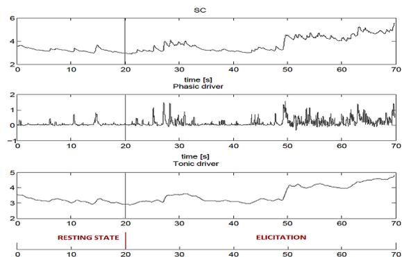
Fig. 3: Example of decomposition analysis. In the upper figure the row SC signal is shown. The lower figures report the deconvoluted tonic and phasic driver signals during resting and elicitation phase.
