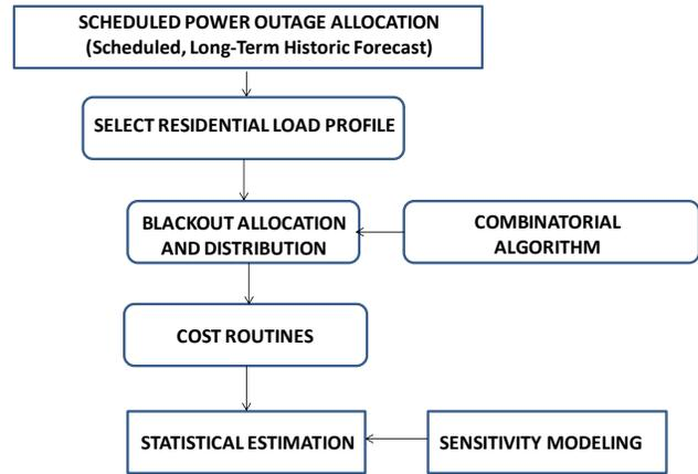
Figure 2(a). Fast Blackout Assessment Tool Architecture.
