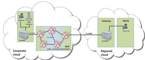
Figure 5. G2MPLS based simplified communication
