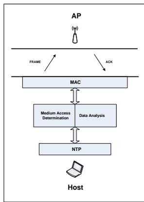
Figure 3. MAC to NTP interface module
