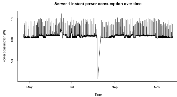
Figure 1. Instant power consumption over time (Server 1)
