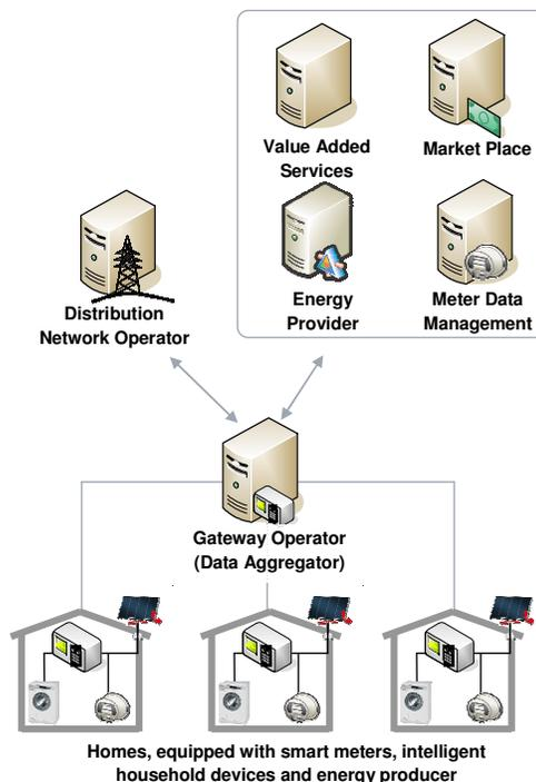
Figure 1. Connection of households to the smart grid
