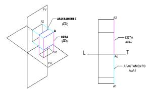
Figure 2. Afastament and cota's point located in first dihedral. Spatial representation and Epure.
