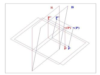
Figure 5. Stereoscopic drawing of (P) point projections on the horizontal and vertical planes.
