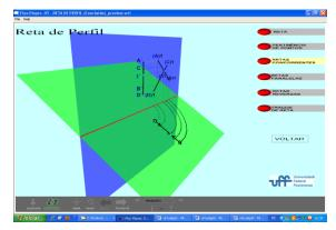
Figure 13. Revolution of the horizontal plane on the vertical plane to obtain the "Epure".
