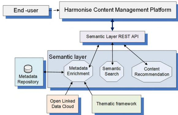
Figure 2. The logical architecture of the SLH
