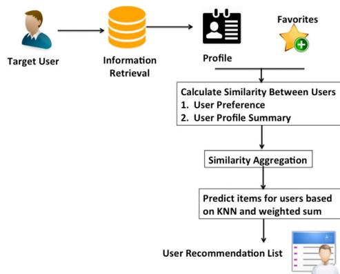
Figure 4. Overview of the CRS Algorithm
