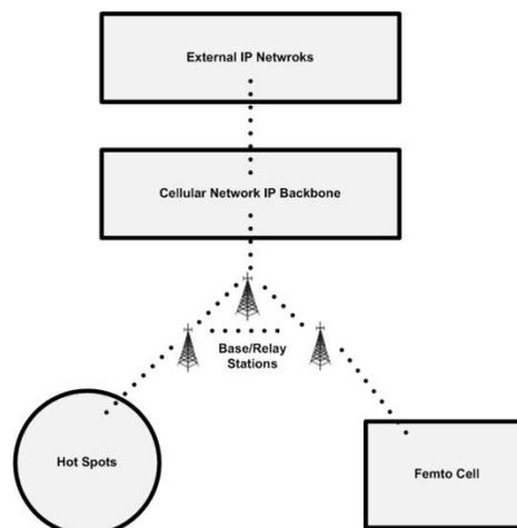
Fig. 4. Basic Architecture of Cellular Network
