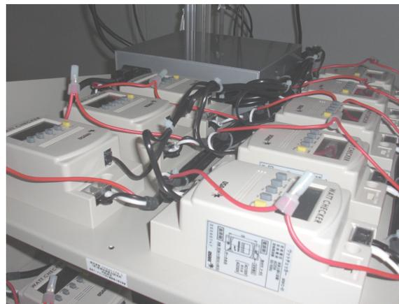
Figure 4. Power Measuring System
