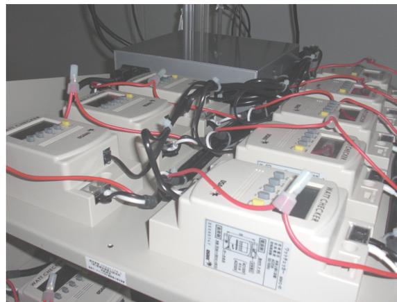
Figure 4. Power Measuring System
