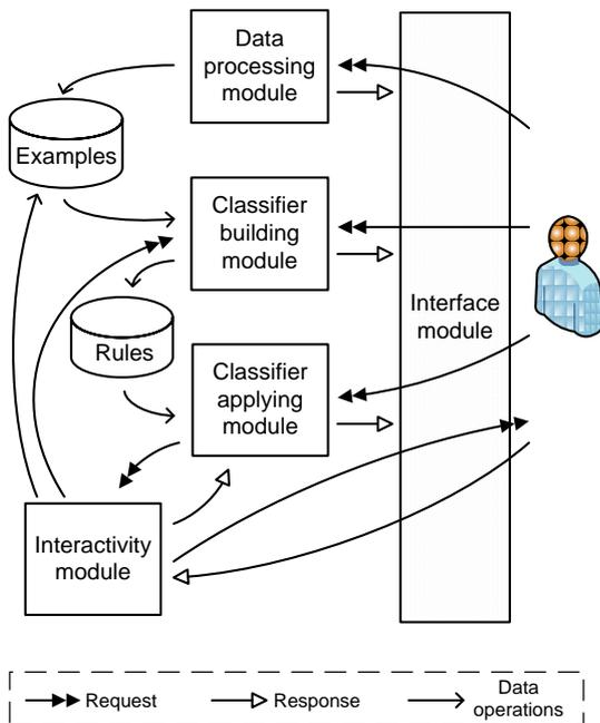
Fig. 14. Functioning of the interactive classification system
