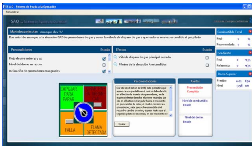
Figure 2. Adaptive user interface layout: adaptive content area on the right side and standard display area separated to minimize impact on user
