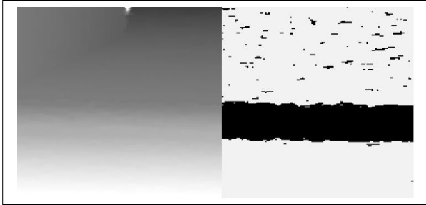
Figure 1. Left side: Depth values from the Sensor in grayscale (White near, dark grey far away) with a 10mm doorstep in a distance of 80cm, right side: Visualisation after ground subtraction and convert to a binary image of depth values with the RMS as threshold
