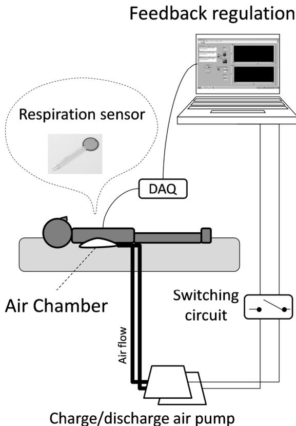
Figure 2. Schematic diagram of our respiration-posture feedback system.
