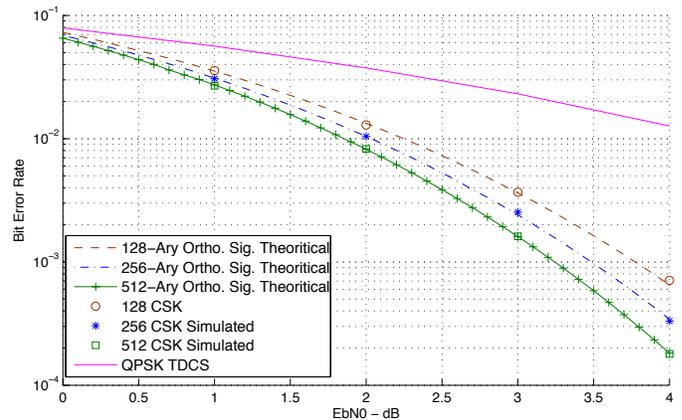
(b) BER performance of TDCS System using  $M_{\text{CSK}}$ -Ary CSK Modulation with  $M_{\text{CSK}} \geq K_{\text{used}}$
