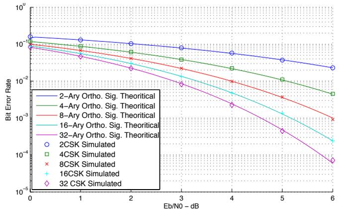
(a) BER performance of TDCS System using  $M_{\text{CSK}}$ -Ary CSK Modulation
