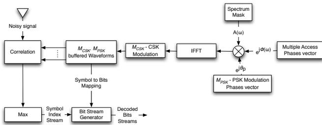
Figure 2. TDCS Optimum Receiver
