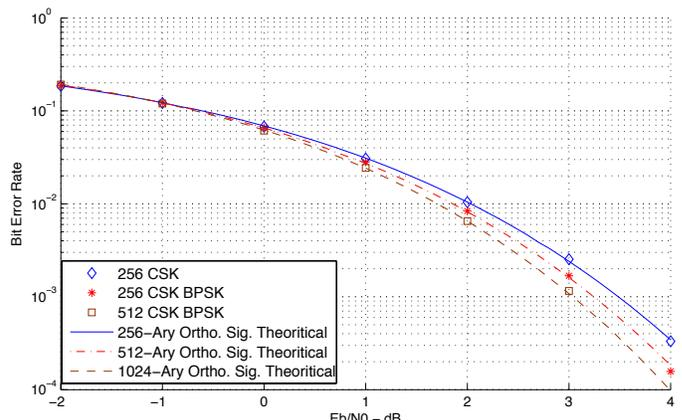
(c) BER performance of TDCS system using an Antipodal  $M_{\text{CSK}}$ -Ary CSK Modulation
