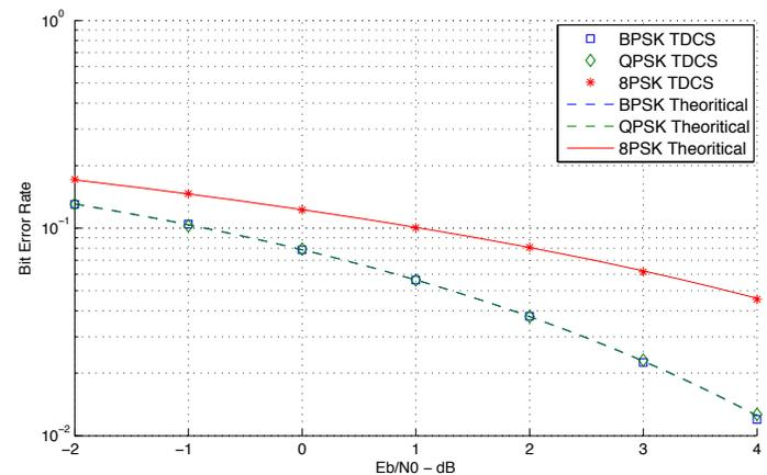
Figure 4. BER performance TDCS using  $M_{PSK}$ -Ary PSK Modulation
