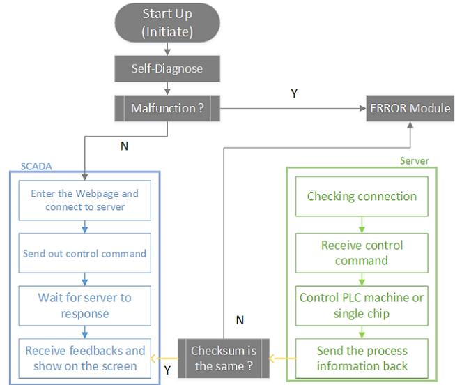
Figure 5. PLC’s working process
