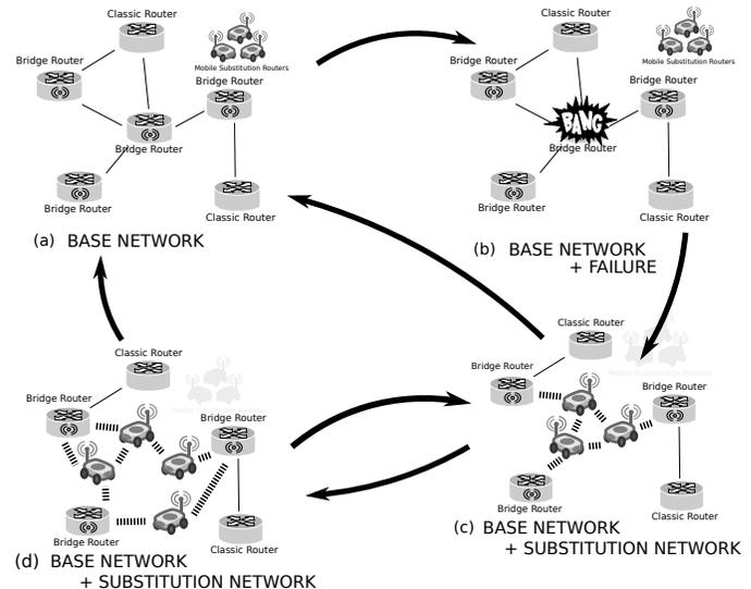
Fig. 1. Typical use case for a base network and a substitution network.
