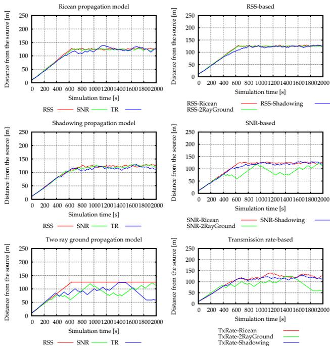
(a) Comparison of the link parameters (b) Comparison of the each parameter for each propagation model.
