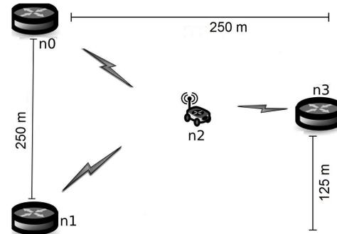
Fig. 7. Two sources, one destination, and one mobile router scenario.
