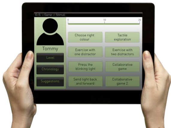
Figure 7. The screen-based interface that would allow the therapist to load and configure new play scenarios, as well as to keep track on the progress of each subject.
