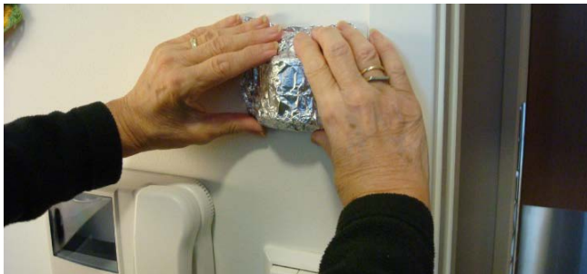
Figure 1. Covering a sensor with tinfoil (Photo: S. Finken [1])
