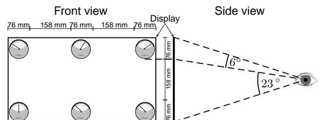
Figure 1. Task configuration with six gauges (reconstructed from [5]).
