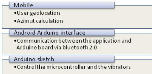
Figure 4. Structure of the system's applicative part.
