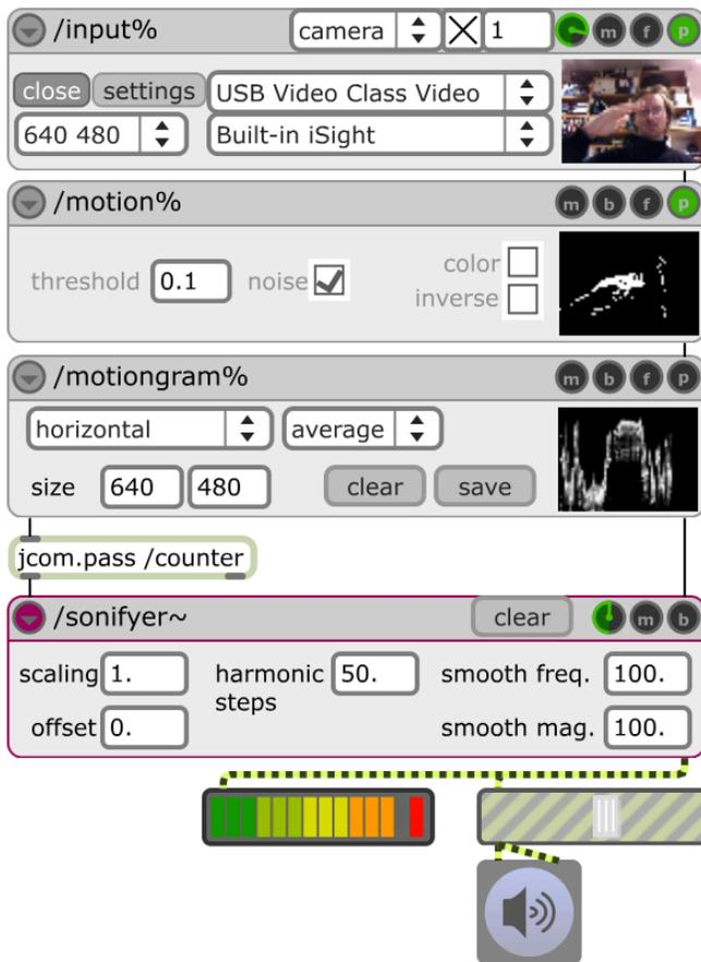
Figure 4. From the help patch of the `jmod.sonifyer~` module. The video input module is connected to a module creating the motion image and then to the motiongram module. Finally, the output motiongram is sent to the sonifyer module for the creation of sound.
