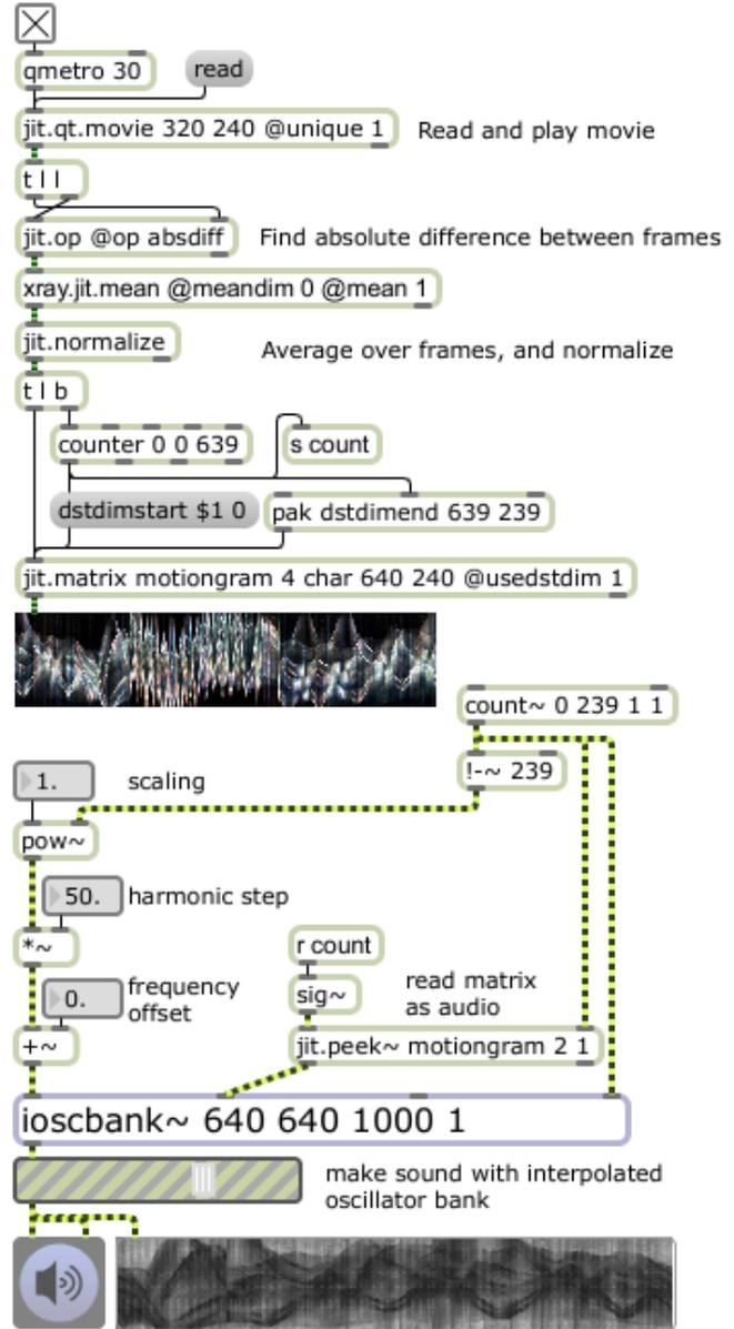
Figure 3. A minimal Max implementation for generating the sonification from video input. The oscillators are created in the `ioscbank~` object, and Jitter matrix data is converted to an audio signal with the `jit.peak~` object.
